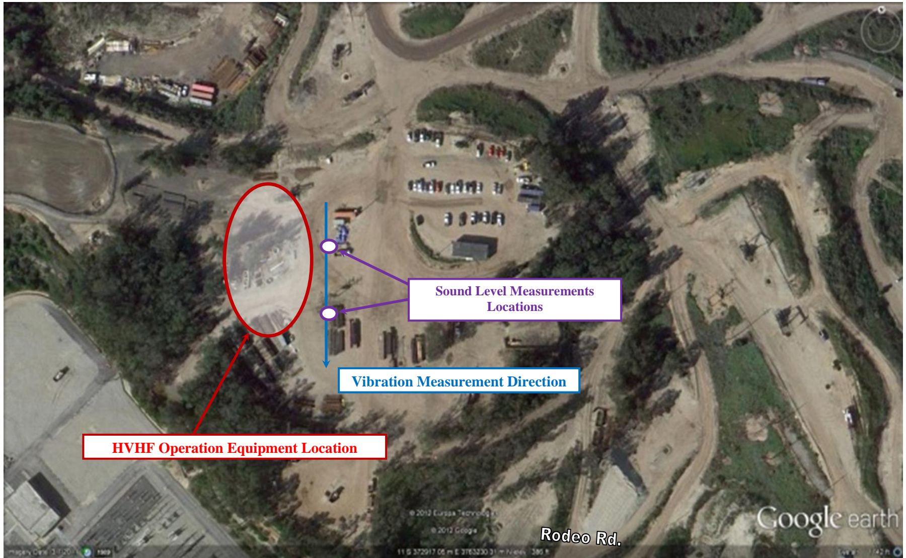
HVHF Operation Vibration Measurement Direction at VIC1-635 site
