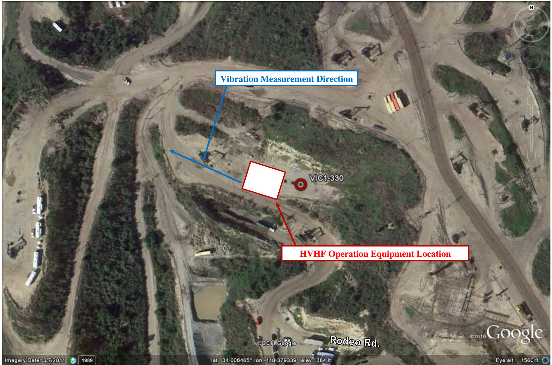
HVHF Operation Vibration Measurement Direction at VIC1-330 site
