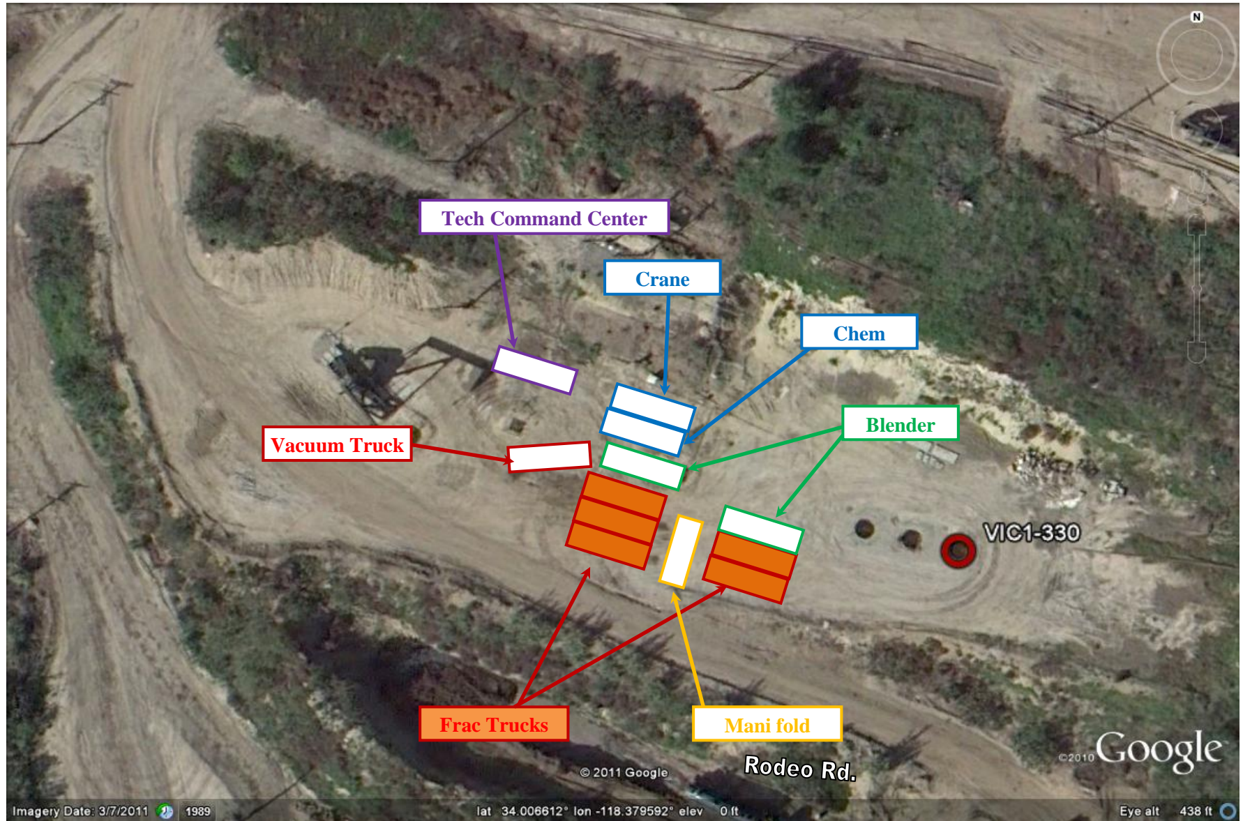
HVHF Operation Equipment Layout at VIC1-330 site
